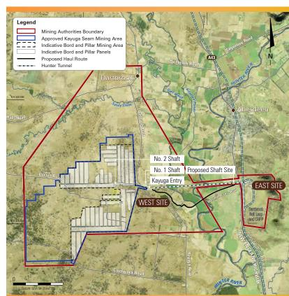
Figure 1 Conceptual Modification Layout
