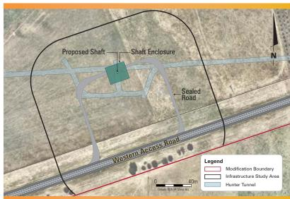
Figure 2 Conceptual Layout of New Shaft Site
